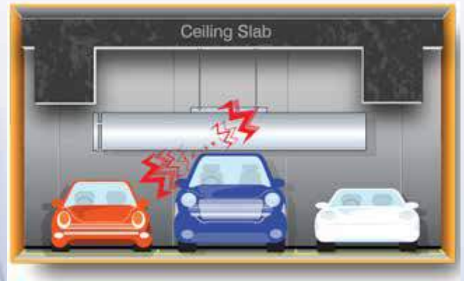
Figure 8(b). Insufficient clearance
