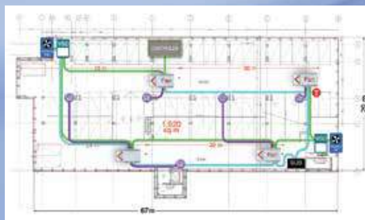
Figure 12. Fan sizing and placement example
