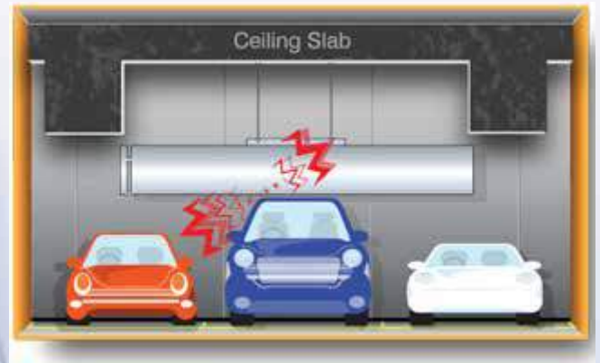
Figure 8(b). Insufficient clearance
